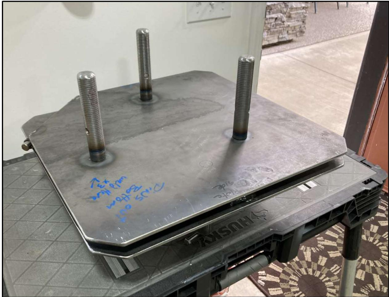
A hinge-plate assembly was fabricated such that it could be inserted between the tower base to tower sections.
