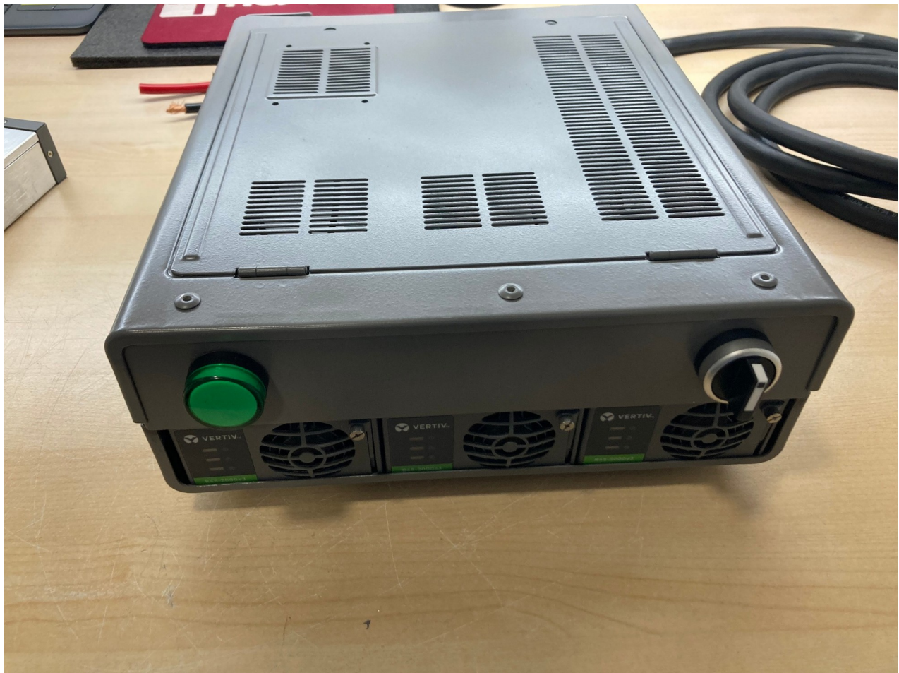
Figure 1 Completed VE6HQ Vertiv R48 Three-Rectifier Power Supply
